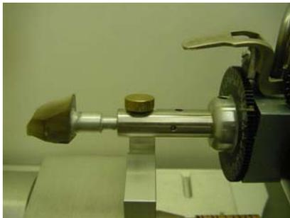
On the Mast, set the Quill angle at about 90+ degrees. Raise the height position of the Quill so that as the Mast is advanced forward (which is what will happen next) the Quill will pass over the top edge of the Plate. Using the X adjustment knob, advance the Mast toward the Alignment Plate until the front end of the Quill is a small amount higher than the top edge, and perhaps a quarter inch past the back face of the Alignment Block - as shown.
