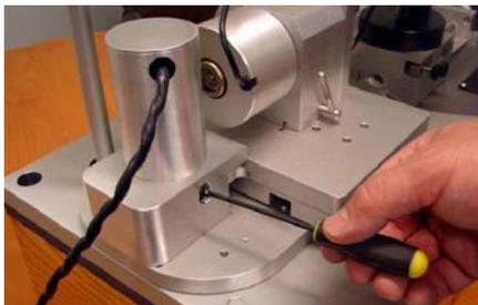
The setting is performed by engaging a screw that is visible in the side “window”, as shown. The adjusting screw rotates with the rotation of the motor – and to perform the adjustment, obviously, the head of the screw must be visible (and so, reachable) in the window. A slow jogging of the motor can bring the head into view, or...
