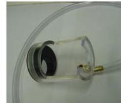
Slip the black piece over the Spindle and set it into the hole – it's a “slip fit” (but fairly snug).
