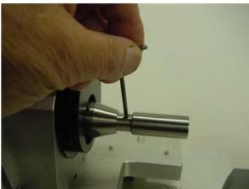
the cylindrical tool is inserted – and, in turn, locked in place with the setscrew in the Adapter.
