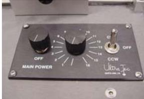
**4.1.1 Control of Tool-drive Motor** The right-side Switch is a two-way ON-OFF toggle for the Tool-drive Motor. It has a choice for motor direction – UP for clockwise (CW) rotation of the tool, and DOWN for counter clockwise (CCW) rotation of the tool. The central position of the switch is OFF.
