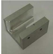
The RF, which completely eliminates Yoke swing, is used for setting the “Home” position. It *can* remain in place for the concave faceting, but, unlike the RC, it does not allow any swing of the Quill, and so inspection is a bit more difficult. Note that inspection can be done by rotating the Quill, and then, re-indexing the Quill position to continue work
