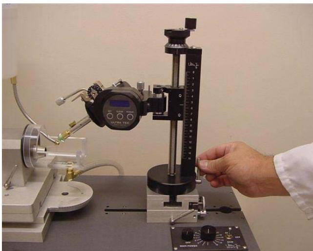
Slide the Mast into the slot in the top plate of the Mounting Block.
