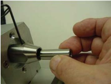
This picture shows inserting an Tool Bushing into the .625 diameter hole of the Basic Adapter (as you can see, the Tool Bushing selected for this photo has a 1/4” hole – selected to accept the particular tool planned for use).
