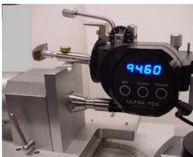
Loosen the Base lock on the Mast (slightly) so that the Mast can be rotated on the Mounting plate, and rotate the Mast so that the Quill (still over the top edge of the Alignment Plate) is to the side of the notch—by perhaps a half inch. Now, lower the Quill position so that it comes to a rest on the top edge of the Alignment Plate, and continue to lower until the angle readout is about 94 degrees – no precision needed (my 94.6 is OK). Disengage the Angle Stop on the Mast – back it off.
