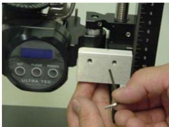
Hold it firmly – tighten the set screws. Feel the Yoke – confirm that it is rigidly held.
