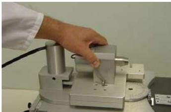
...it can be positioned by pushing or pulling the Tool-drive Motor Plate (it's OK to grip the Motor housing to do this as shown). This method will not work if the head is located, by chance, in a straight line with the reciprocation action (at an extreme of the reciprocation). If that happens, jog the motor so that the reciprocation stroke moves to an about half-way point, and try again.
