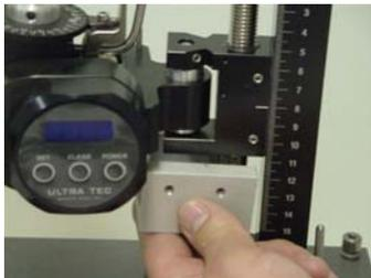
Approach from under the Riser Block. The U cutout clears the Leadscrew. Push up.
