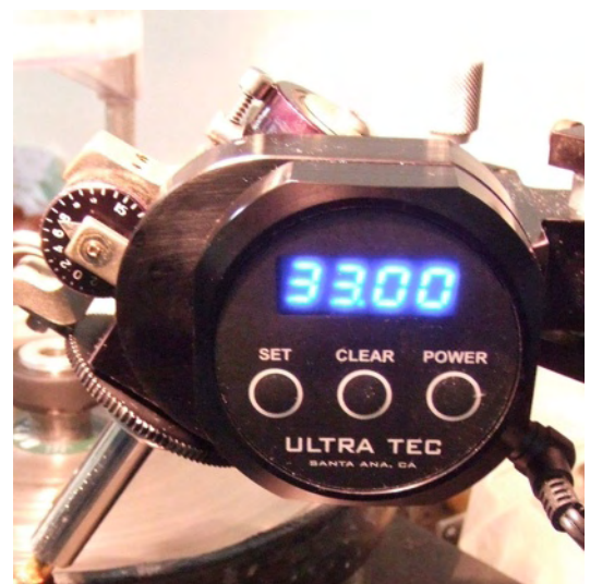
Accurate to 2 decimal points (.01 of a degree)
