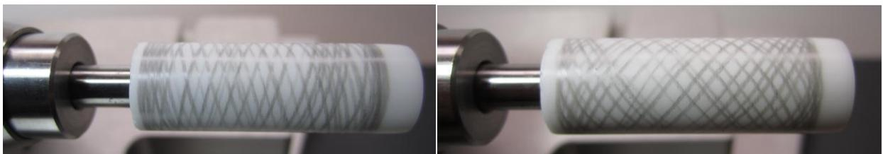
concave facet. Since both the Fantasy and the Concave Machine by Ultra Tec have independent controls for each motor the ratio can be adjusted. For the most effective pattern the oscillating motor control is turned up and the drive motor is turned down. An additional feature of both of these mentioned machines is the ability to adjust the amplitude( distance the mandrel travels).
